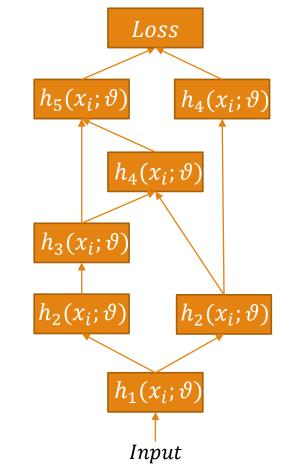
• A neural network model is a series of hierarchically connected functions
